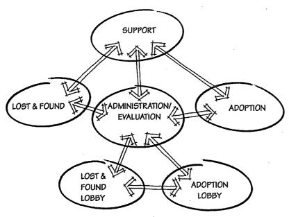
As shelters grow in size, the individual modules that are part of the basic triangular concept expand to include individual rooms for specific functions. Some of the modules, such as administration and evaluation, might actually fracture into two pieces; one devoted to evaluation purposes and the other to support purposes such as food preparation, utility, and grooming.
