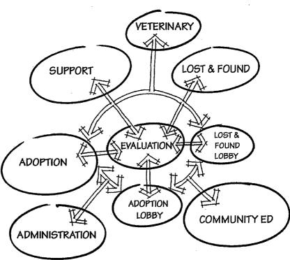
functions. This reduces circulation and duplication of equipment and staff and also streamlines operations. Even in the very largest facilities, it makes sense to create a core area that includes such services as material receiving and shipping, storage, food prep, utility, laundry, lockers, and grooming.
