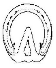
The nail clinches should be evenly spaced and in a level straight line.
